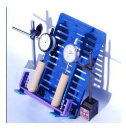
Fig. 1: Core shrinkage measurement fixture
