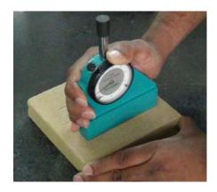
Fig. 2: Mold hardness measurement
