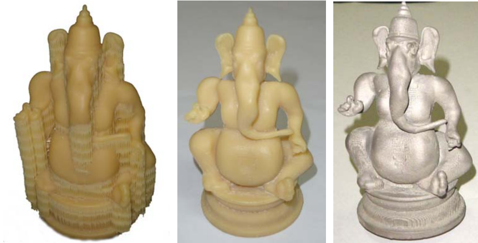
Fig. 5 Physical realisation of Ganesha: wax pattern made by rapid prototyping, followed by support structure removal and investment casting.
