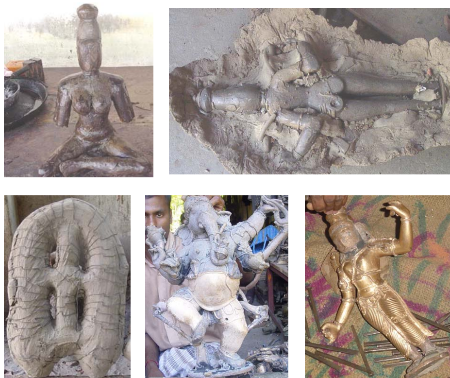
Fig. 1. Ancient lost wax casting method: wax model sculpting, clay covering, wire clasped mould for dewaxing, as-cast Ganesha, and finishing
