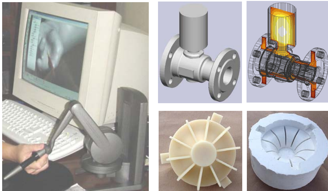
Fig. 2. Some modern technologies relevant to investment casting of complex parts. Left- touch based solid modelling; right top- intelligent feeder design and analysis; right bottom- rapid prototyped wax model and corresponding rubber mould.
