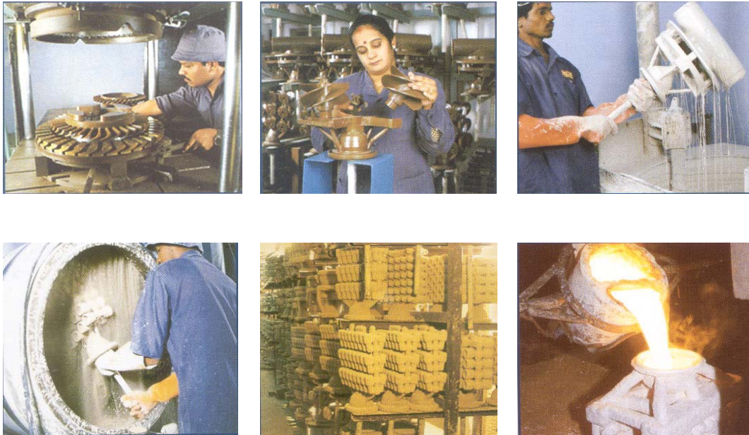
Fig. 2. Industrial investment casting process: wax injection pattern, attaching to gating, dipping in ceramic slurry, sand stuccoing, controlled drying and pouring in hot mould.
