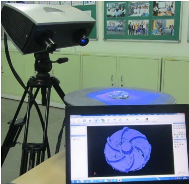
Fig. 9: 3D scanning of impeller casting
