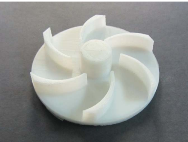
Fig. 6: 3D printing of impeller pattern using RapidBot
