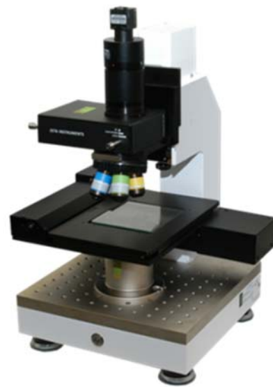
Fig. 11: 3D microscope (Zeta 20) used for surface inspection
