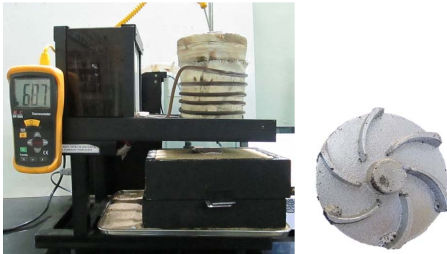
Fig. 8: Metal melting and direct pouring using Melt-IT tabletop furnace
